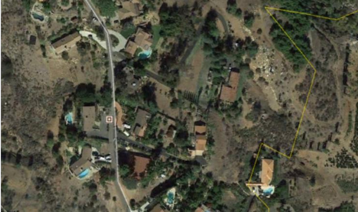
Figure 6. Example of moderate density development. Structures are located on larger properties and include varying levels of ignition resistance and landscape / fuel modification provision and maintenance. This type of development results in a higher wildland exposure level for all homes and does not provide the same buffers from wildfire encroaching onto the site, or starting at a structure and moving into the wildlands as a higher density project.
