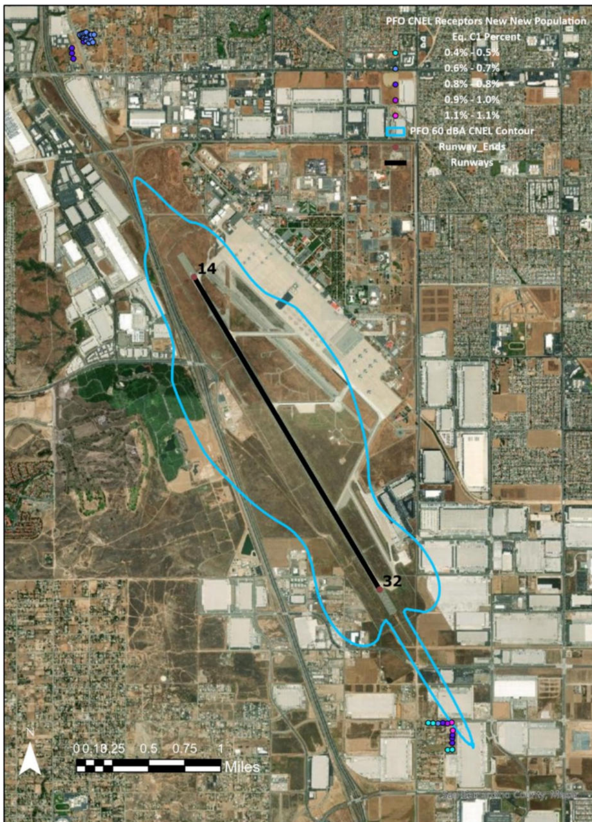
Figure 6C: Preferred Flight Operations CNEL Contour and Percent of New Population Potentially Awakened
