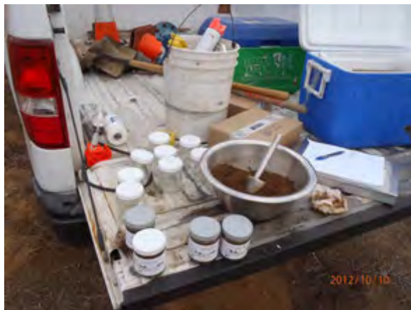
Composited stock pile soil sample collected and delivered to lab with 1/2 the excavation confirmation samples
