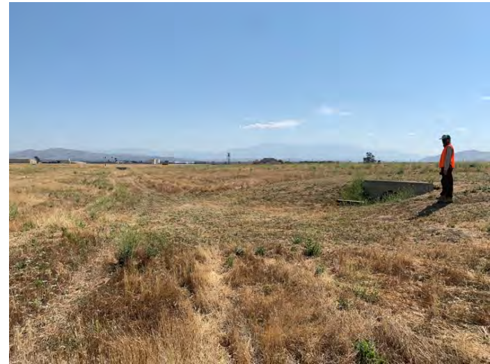
Photo 24. Overview of S-1 showing a second culvert outlet. The area did not display OHWM indicators or a bed and bank. Photo taken facing east (33.878624, -117.250920).
