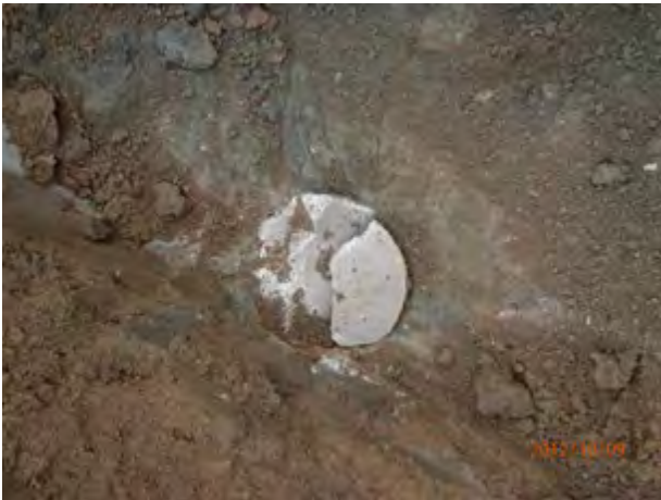
Observed grouted up soil boring penetrating gray soil
