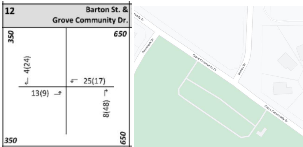
Exhibit 4-3 from Appendix N and a map of the 3-way intersection modeled as a 4-way intersection.
