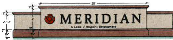
20' Long Major Monument Sign with Wing Walls at Cactus Avenue Site Entry
